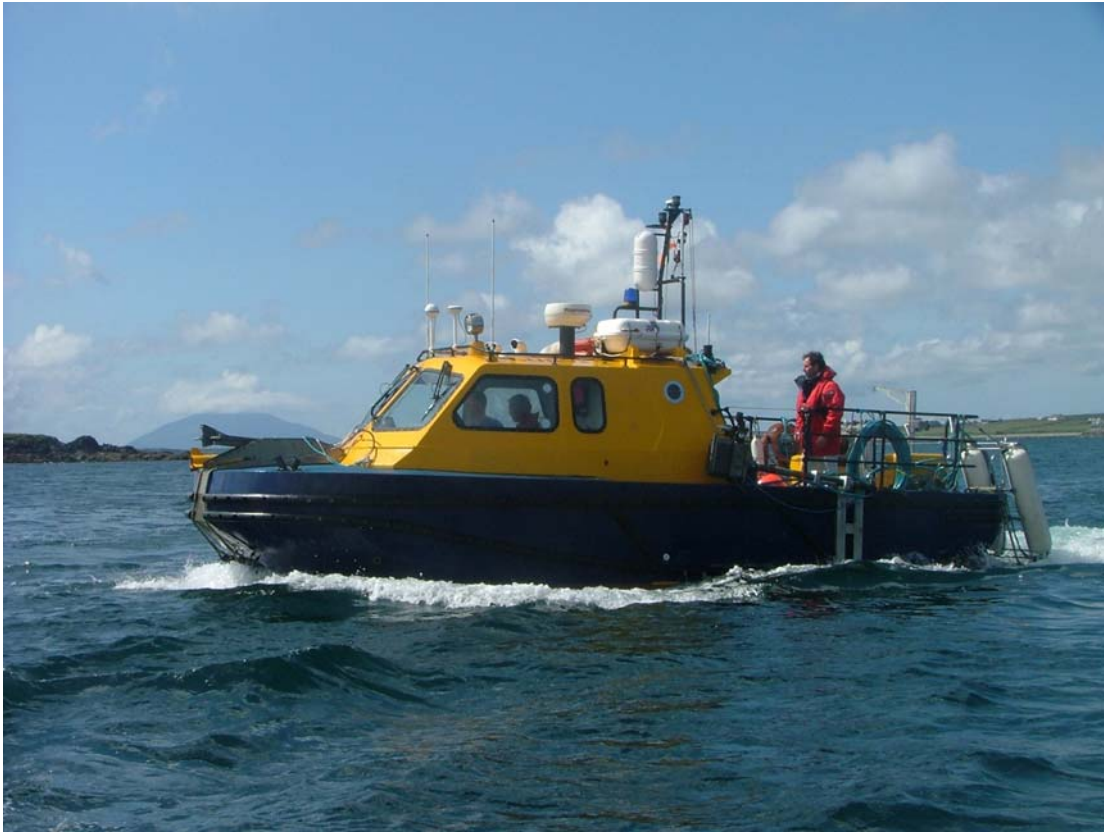
Plate 1. The main survey vessel the Eagle underway. Three sound sources can be seen aboard: (i) side-scan sonar sitting on the bow, (ii) multi-beam echo-sounder positioned horizontally on the port side, and (iii) the boomer resting on the stern in the white fender float.
