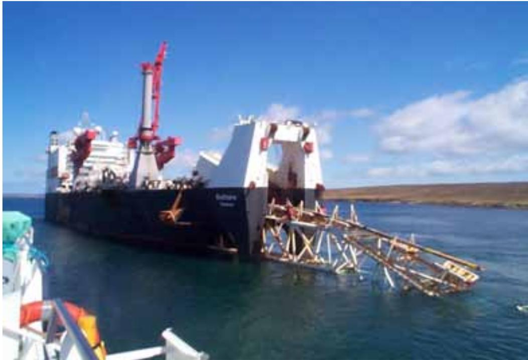
**Plate 6: Dynamically Positioned Pipe Lay Vessel**
