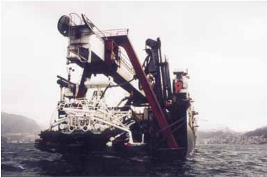
**Plate 7: Trenching vehicle suspended from mother ship**
