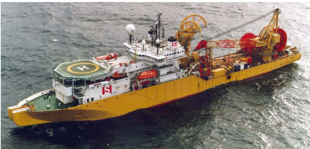
Plate 3.6: Typical dynamically positioned installation vessel (Seaway Eagle)
