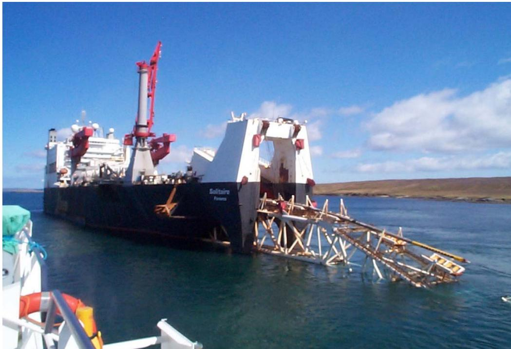
Plate 3.2: Typical pipelaying barge, Solitaire
