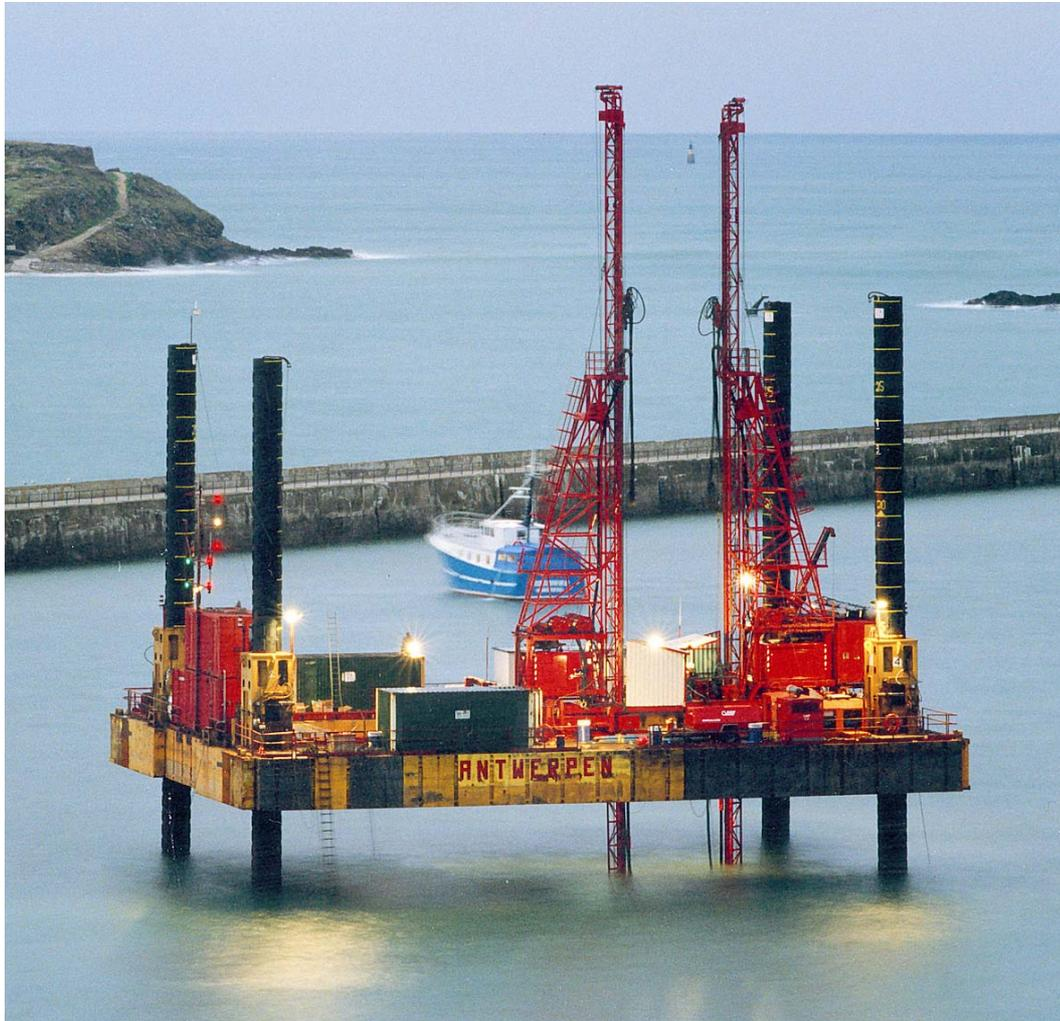
Plate 3.1: Self-elevating platform to support underwater blasting operations
