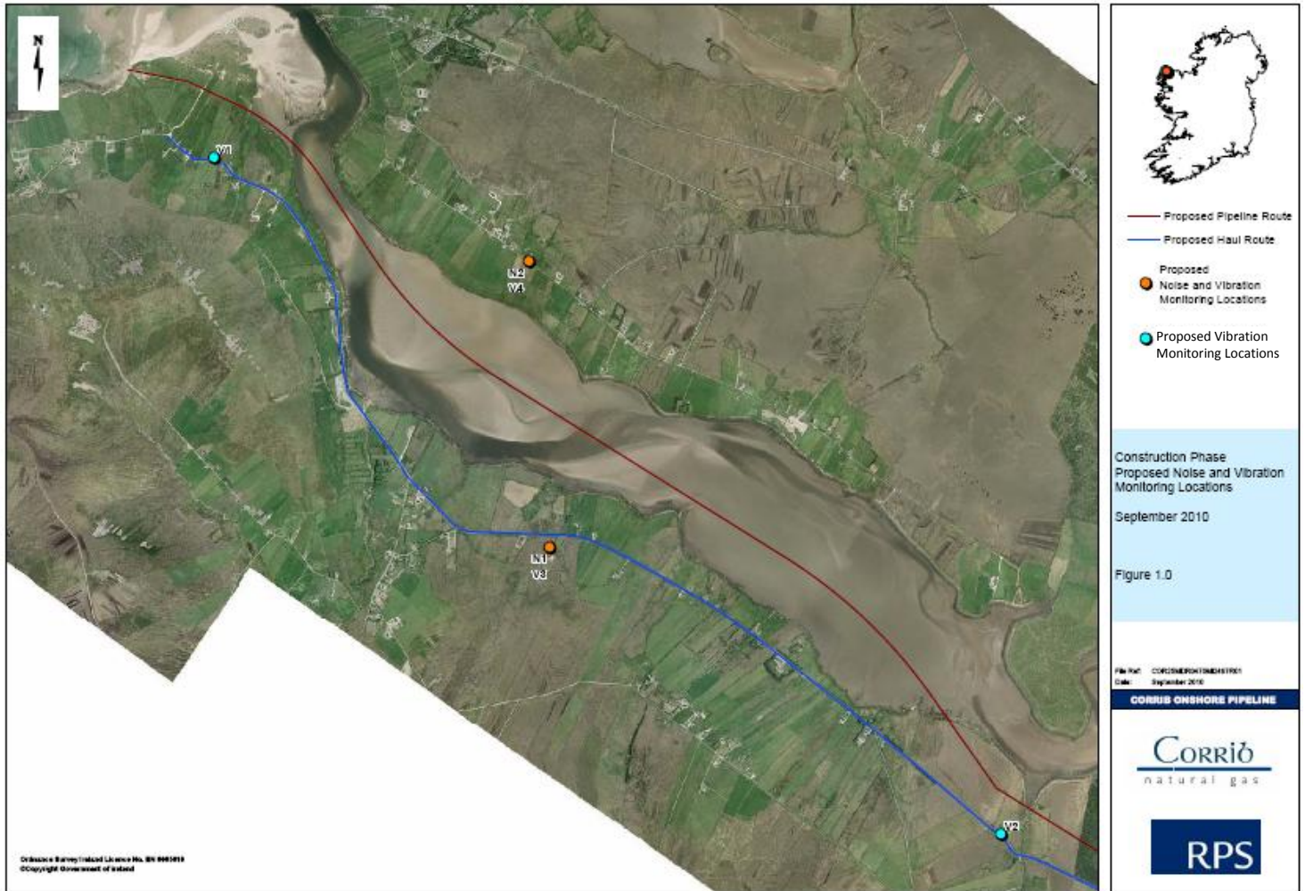
Figure 1. Vibration (and Noise) Monitoring Locations
